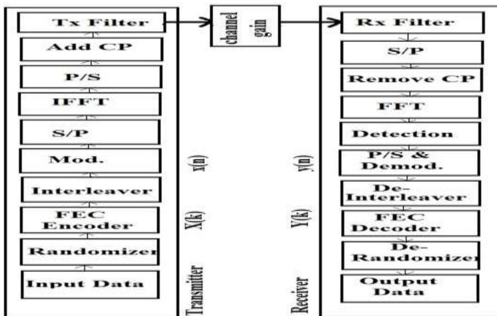
Figure 3: WiMAX physical layer model
